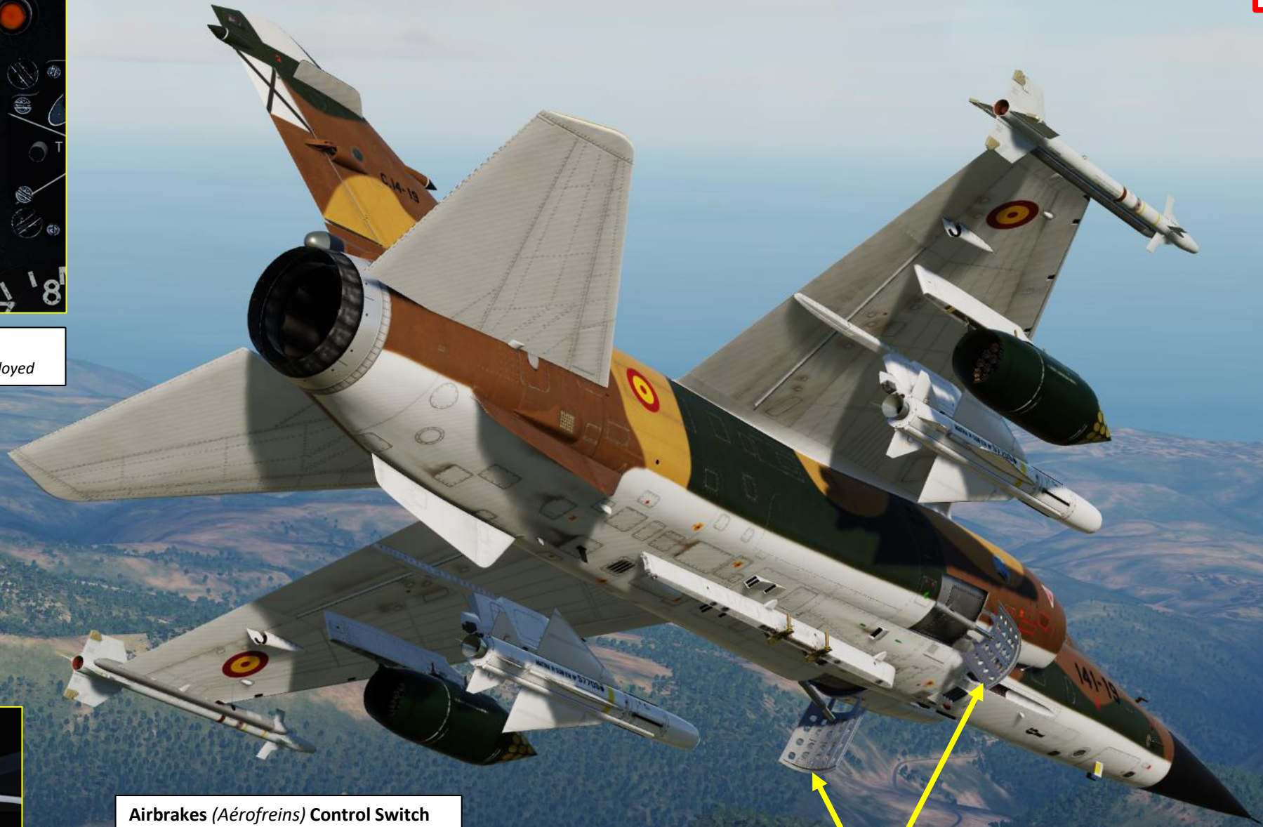
Airbrakes (Aérofreins) • Hydraulically actuated
