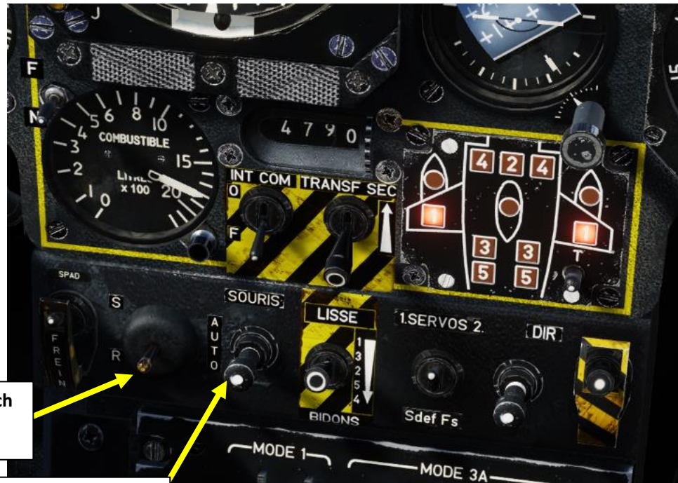
Engine Shock Cone ( Souris ) Pushbutton • Pushed IN: Automatic Control • Pulled OUT: Manual Control Enabled (use the Shock Cone Manual Control Switch)
