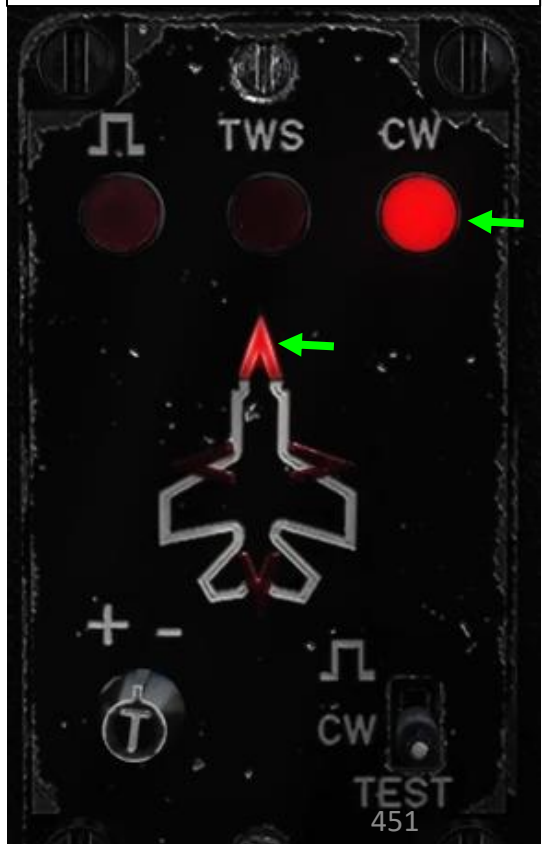
Scenario 4 Continuous wave radar lock, you are locked by a radar which is guiding a missile towards you.
