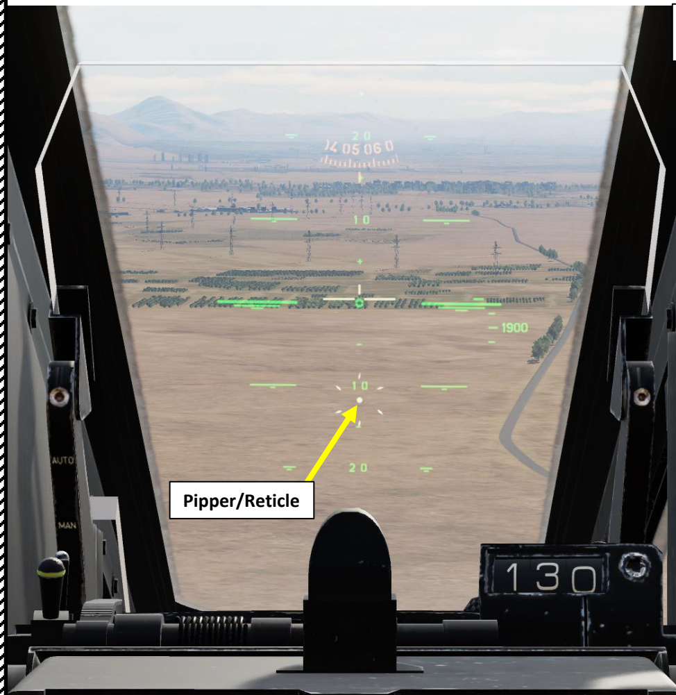
Sight Depression Angle Setting (mRad, milliradians) • Angle is set by Depression Angle Control Wheel
