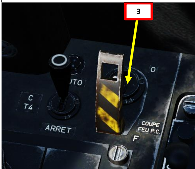
Afterburner (P.C., Post-Combustion) Main Fuel Cock / Fuel Shutoff Valve (Robinet Coupe-Feu) Switch
