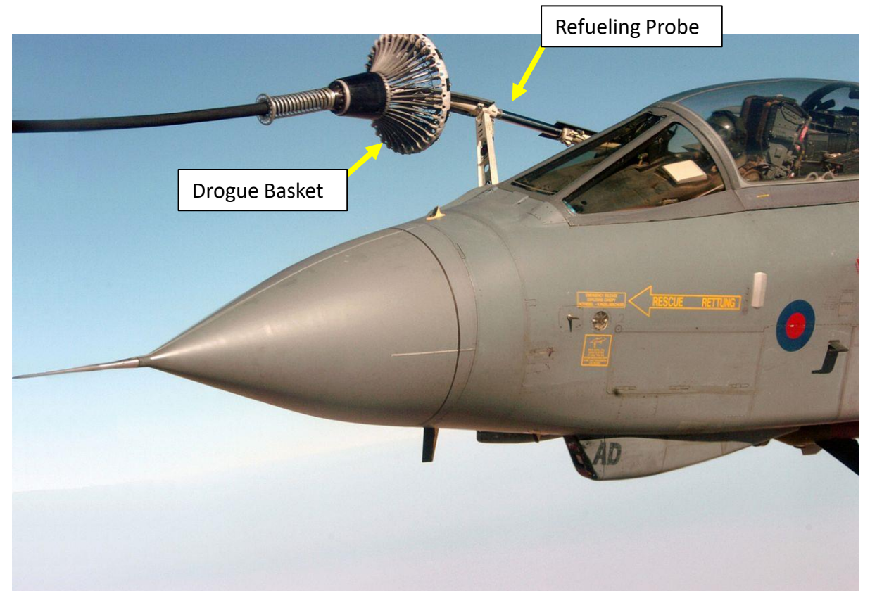
Tornado GR4 being refueled by a Probe-and-Drogue system
