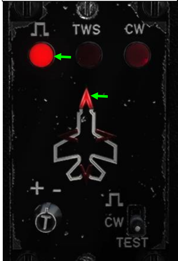
Scenario 2 Pulse modulated radar lock, you are locked by a radar, possibly a fighter aircraft using STT (Single Target Track) mode. Expect a missile shortly.
