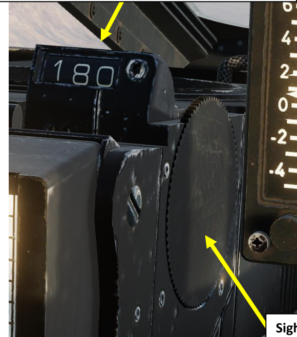
Sight Depression Angle Setting (mRad, milliradians) • Angle is set by Depression Angle Control Wheel
