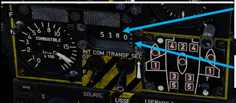
Fuel Remaining Indicator (Liters) • Indicators needs to be set every time a refueling occurs using the Fuel Quantity Reset Thumbwheel.
