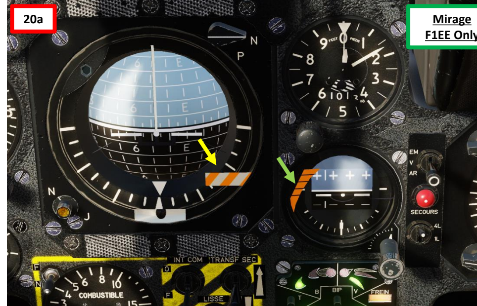
Standby Artificial Horizon Uncage & Aircraft Symbol Adjustment Control
