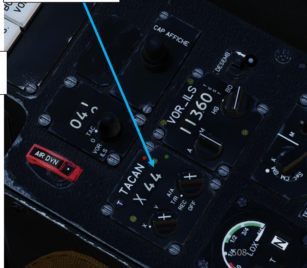
TACAN Frequency/Channel Control Panel
