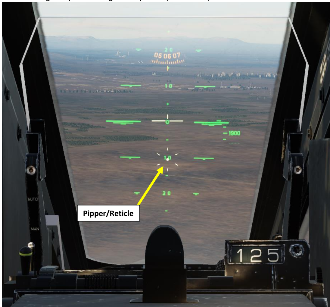
Sight Depression Angle Setting (mRad, milliradians) • Angle is set by Depression Angle Control Wheel
