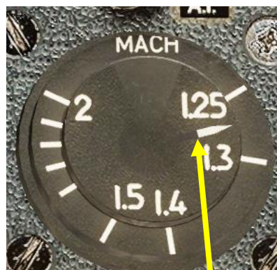
Engine Shock Cone ( Souris ) Position Indicator • Needle indicates the position of the shock cone • The Mach scale indicates the shock cone position recommended for a reference airspeed
