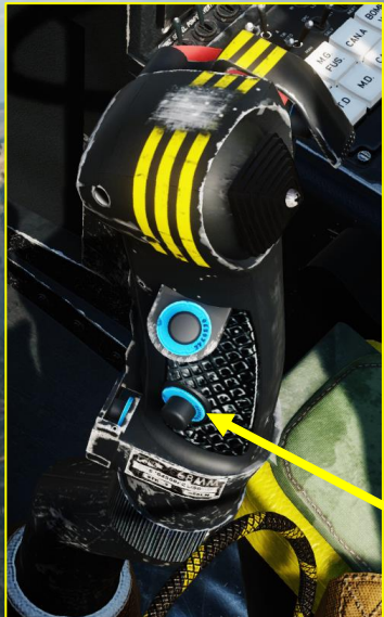
Search Light Control Button ( Phare de Police ) • Press to turn on Search Light
